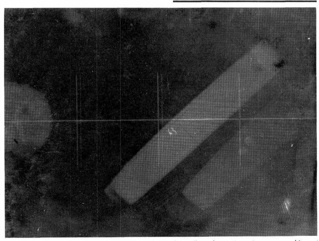
FLASH X-RAY shows the oblique angle of the explosive-driven flyer plate in its trajectory toward impact on the target fuze (at left). White lines are lead wires used as reference points. This testing technique, providing high-velocity impacts, is used in conjunction with rocket sleds which provide lower velocity testing.
